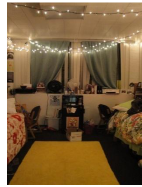
Non-flame resistant curtains and lights not flush with the wall
